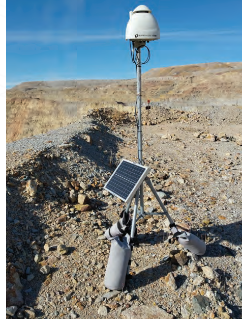
Air quality monitoring unit at Pinto Valley
