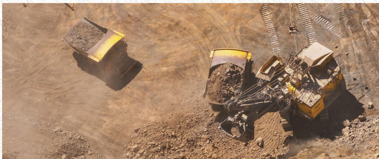
Electric shovel at work, Mantoverde
