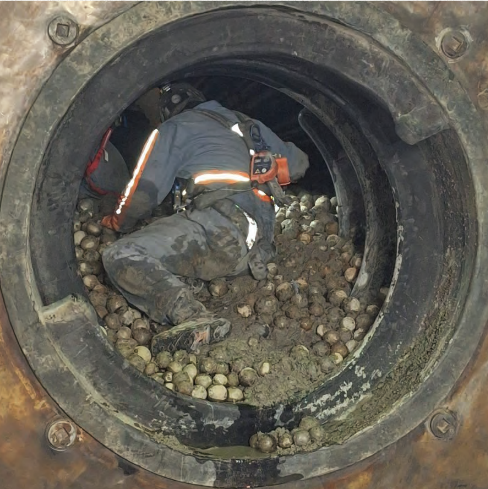
Ball mill maintenance at Pinto Valley
