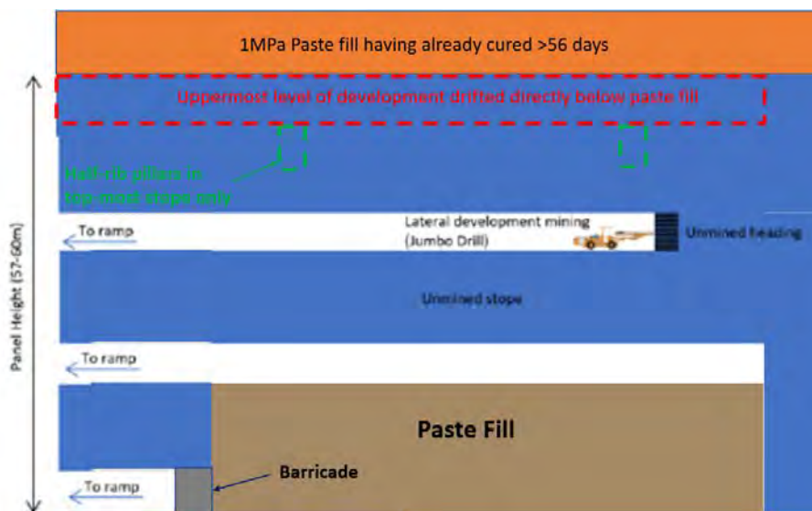
Figure 16-2: Single Vein Longitudinal LHOS Mining Method Diagram Mining Under High Strength Paste Backfill
