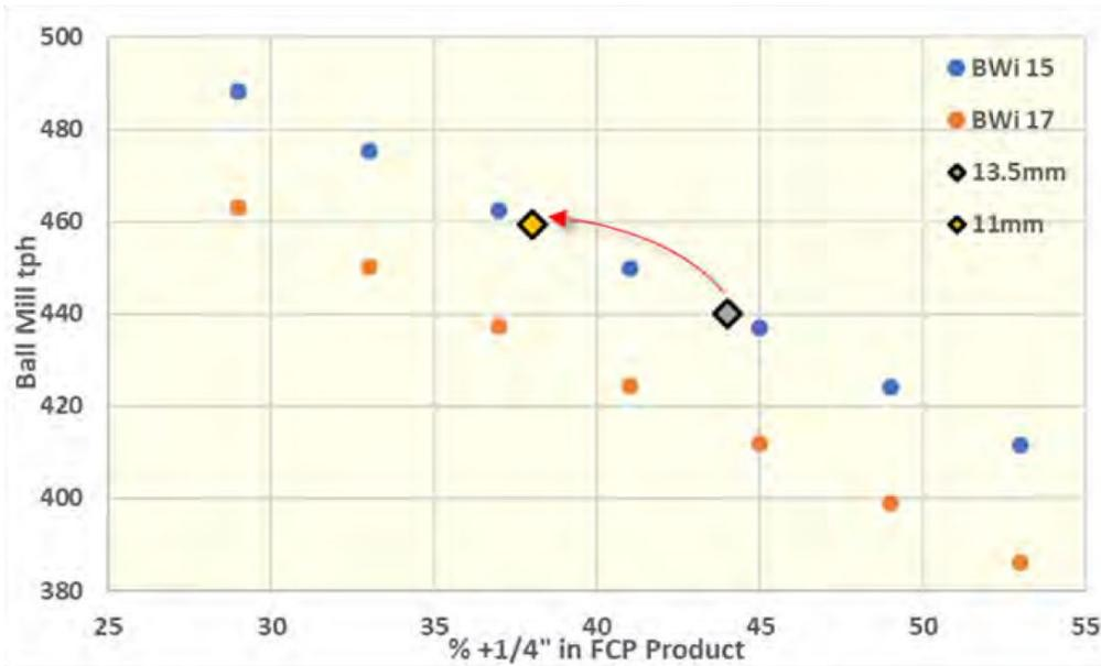
**Figure 13-4: Estimated Effect of Fine Screen Panels On Ball Mill #2 Throughput**
