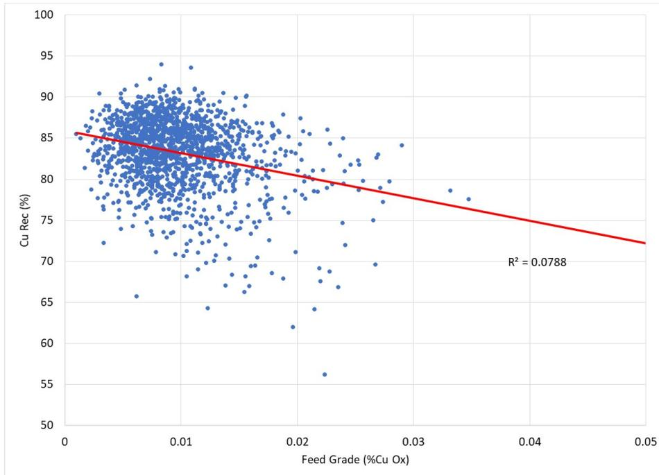
**Figure 13-13: Final Copper Recovery and Feed Grade (Cu Oxide)**
