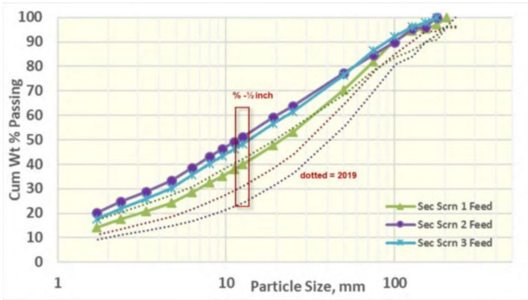
**Figure 13-1: FCP Feed Size – 2020 and 2019 Surveys**
