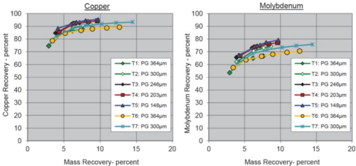
**Figure 13-17: The Effect of Primary Grind Sizing on Copper and Molybdenum Recovery**
