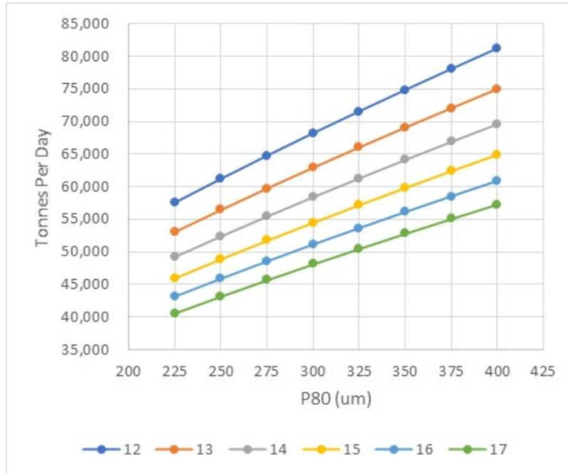
**Figure 13-9: Mill Throughput At Various Work Index and Product Sizes**
