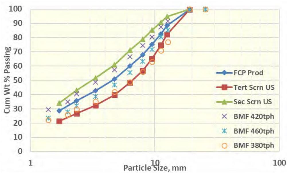
**Figure 13-3: Comparison of Ball Mill Feed Size Vs. FCP Range Of Products**
