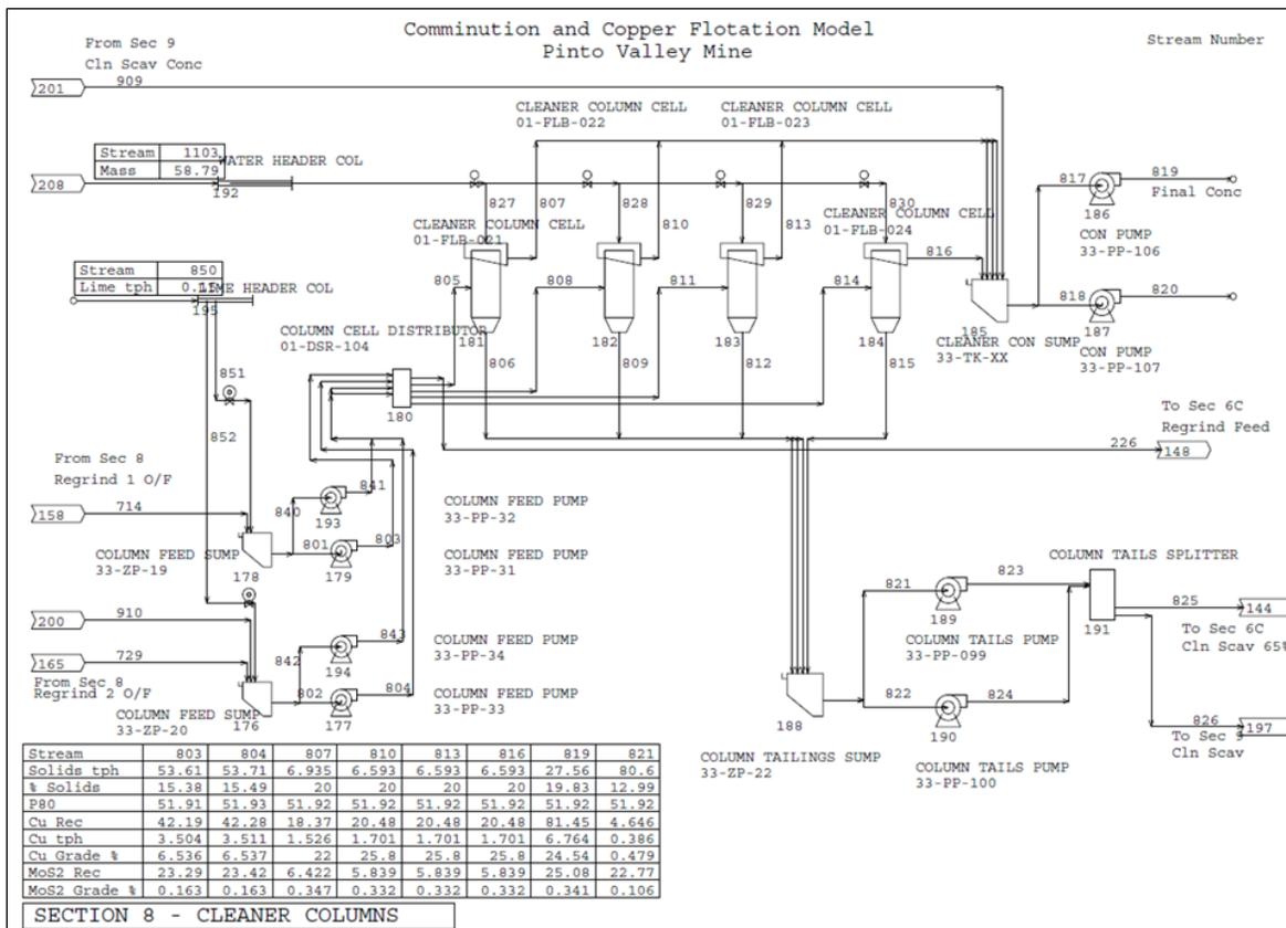
Figure 13-19: MetSim™ Cleaner Flotation Model
