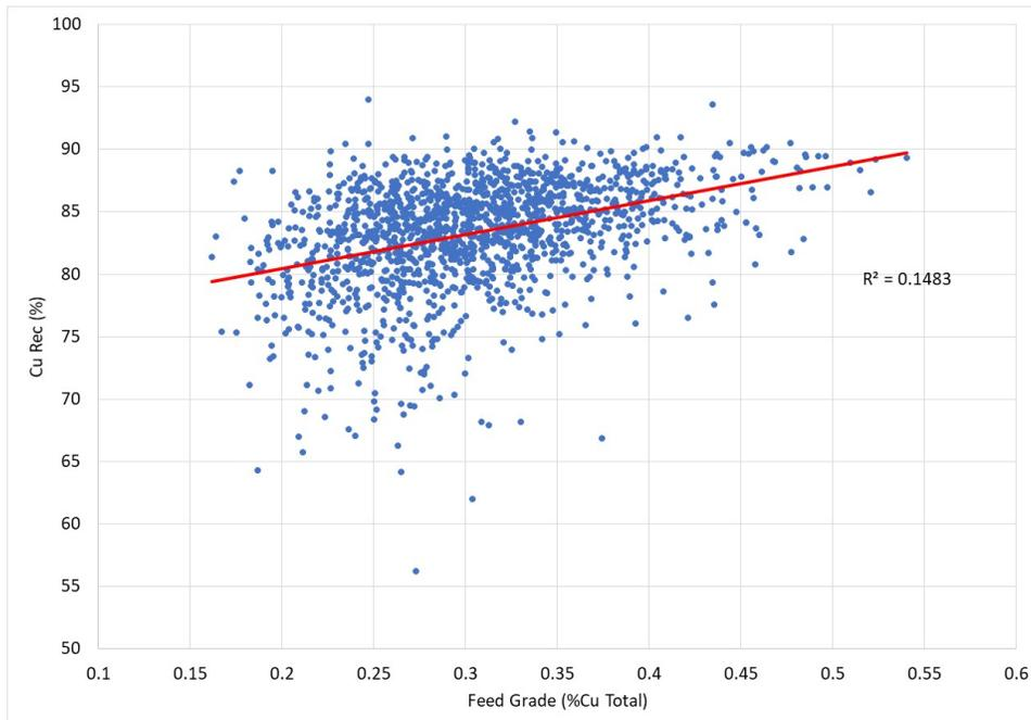
**Figure 13-12: Final Copper Recovery and Feed Grade (Cu Total)**
