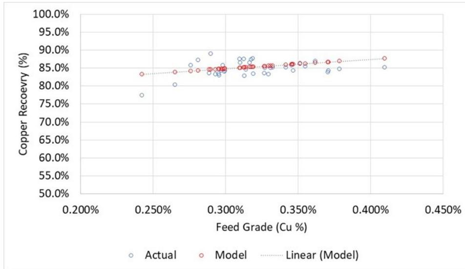
**Figure 13-20: Actual and Model Copper Recovery**
