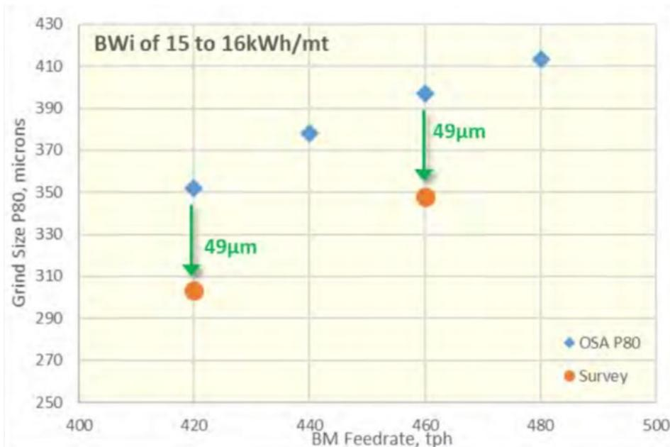
**Figure 13-5: Comparison of On-stream Analyzer Sample P80 Vs. Cyclone Overflow P80 Values**
