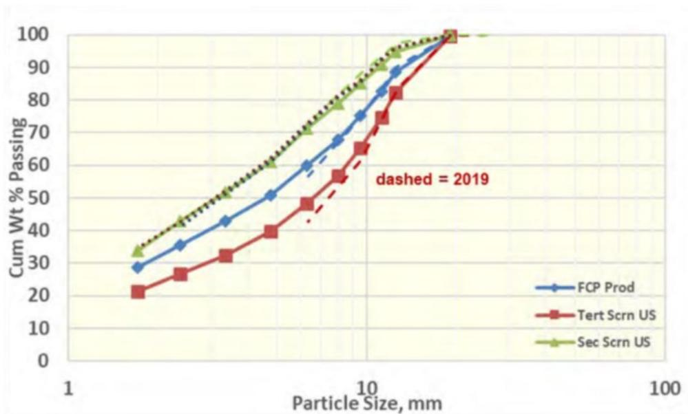
**Figure 13-2: FCP Feed Size – 2020 and 2019 Surveys**
