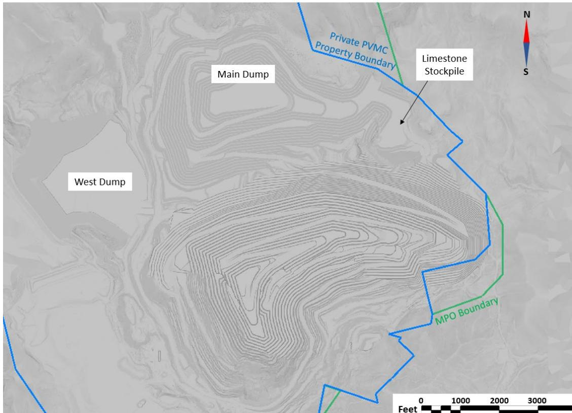
**Figure 16-8: Ultimate PV3-2021 Configuration for Open Pit and Waste Dumps**
