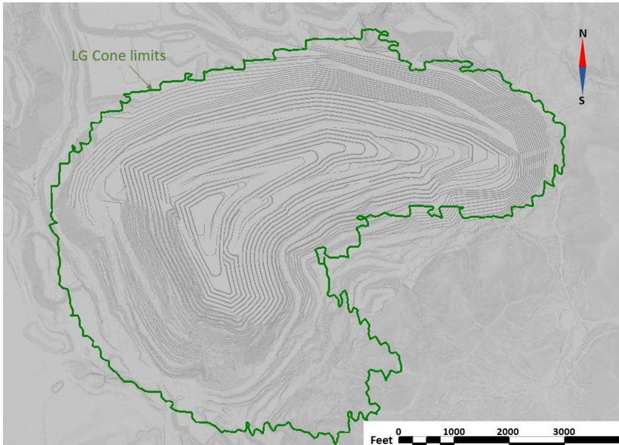
**Figure 15-2: Plan view of Mineral Reserves Pit Design compared to limit of Lerchs-Grossmann at \$3.00/lb Copper**
