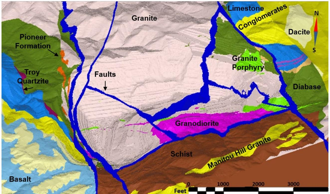
**Figure 14-8: Lithology and Fault Surfaces of the Current Pit Topography to March 31, 2021 (oblique view looking north) (source: Kirkham, 2021)**
