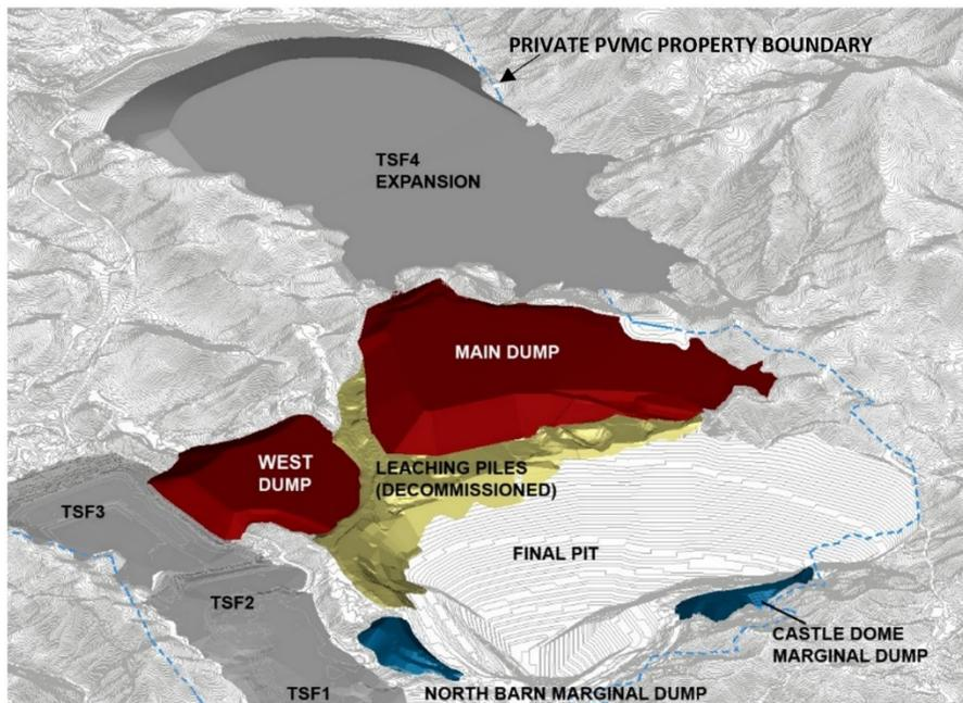
**Figure 20-1: Perspective view looking north, -30 degrees at planned LOM waste rock, leaching, and tailings facilities. Future decommissioned LP (gold), existing and expanded tailings (gray), marginal grade dumps (blue) and planned LOM waste rock (red)**
