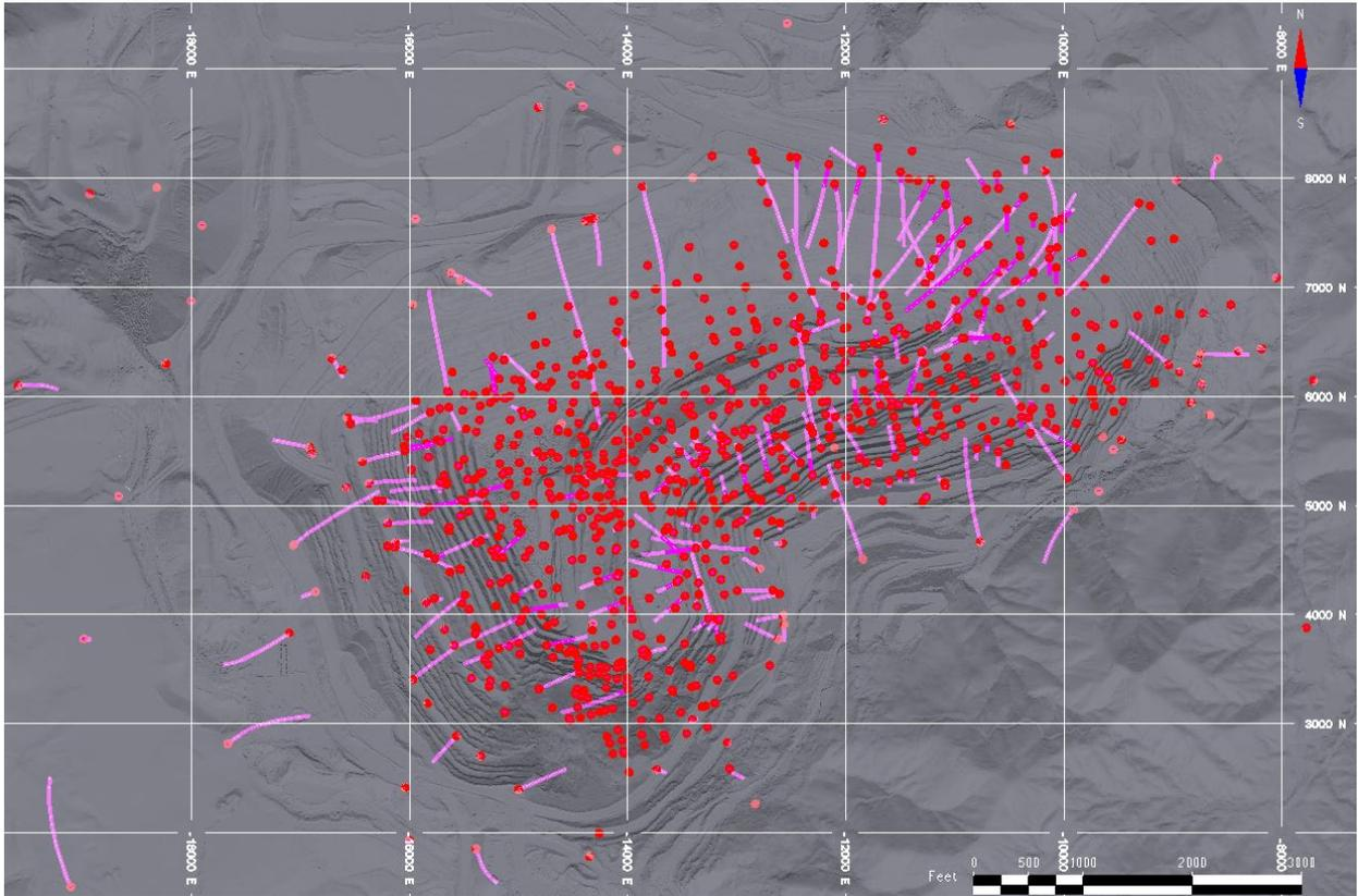
**Figure 14-1: Plan View Showing Drillholes Used with December 31, 2020 Topography (source: Kirkham, 2021)**
