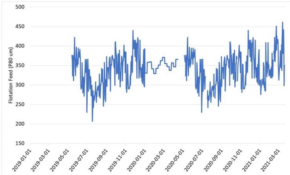
**Figure 13-14: Flotation Feed P80**
