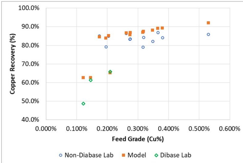
**Figure 13-21: Actual and Model Copper Recovery with Diabase**
