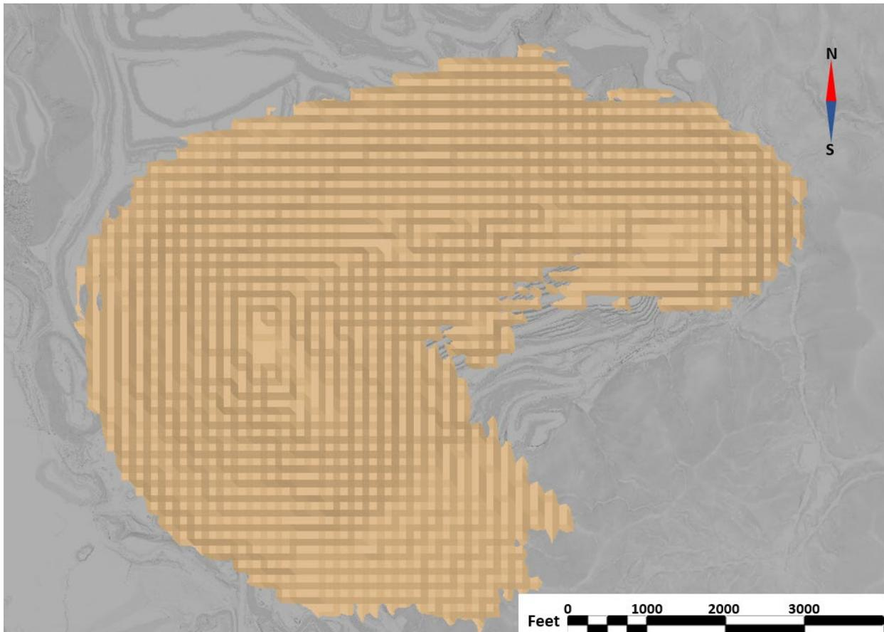
**Figure 15-1: Plan view of Lerchs-Grossmann Optimization at \$3.00/lb Copper (tan), used as Guidance for Phase Design.**
