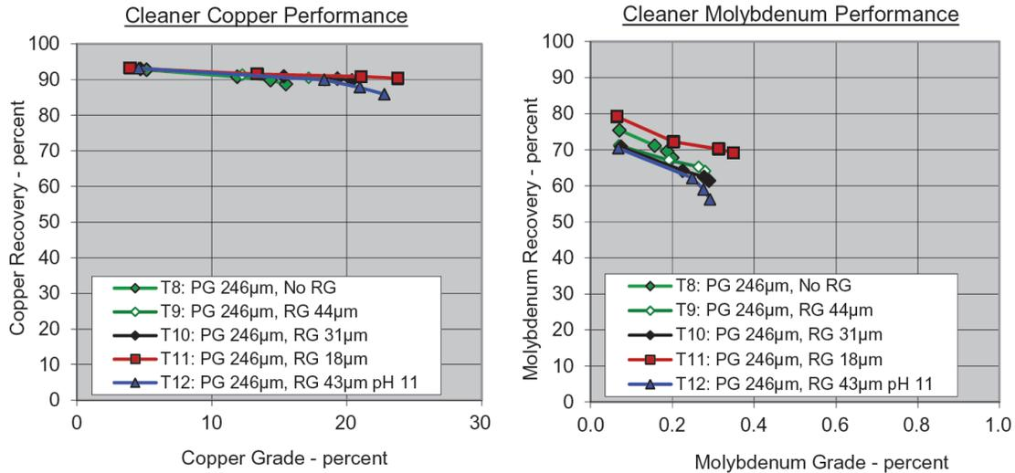
**Figure 13-18: The Effect of Regrind Sizing on Copper and Molybdenum Recovery**
