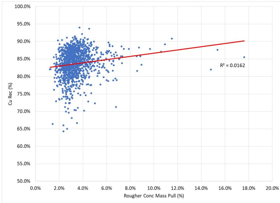
**Figure 13-11: Final Copper Recovery and Rougher Mass Pull**
