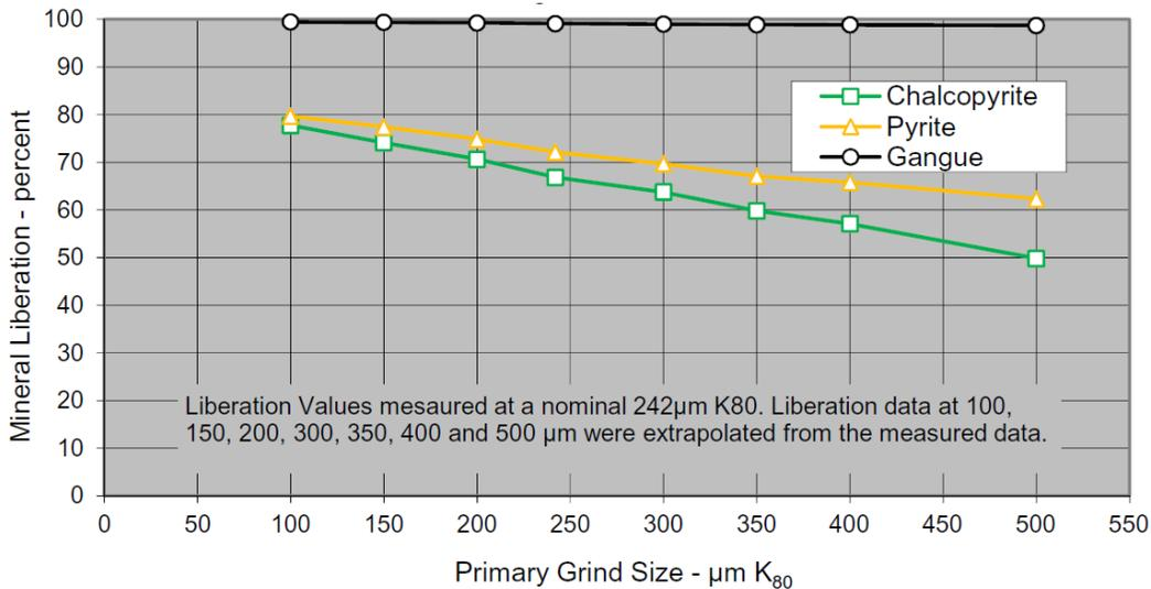
**Figure 13-16: The Effect of Primary Grind Sizing on Mineral Liberation - Rougher Feed**
