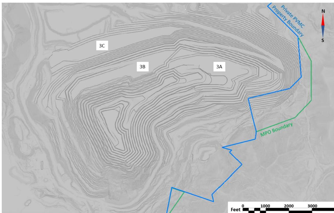
**Figure 16-5: Planned Open Pit Position at end of 2030**
