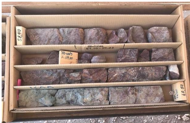
Figure 11-2: Drill Hole DD0013, Half Cores from 58.4 m to 60.5 m
