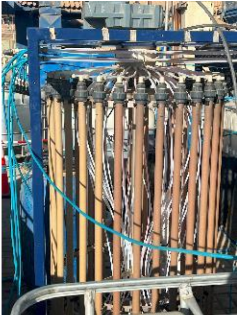
Figure 13-10: Cobalt Loading onto BPA resin.
