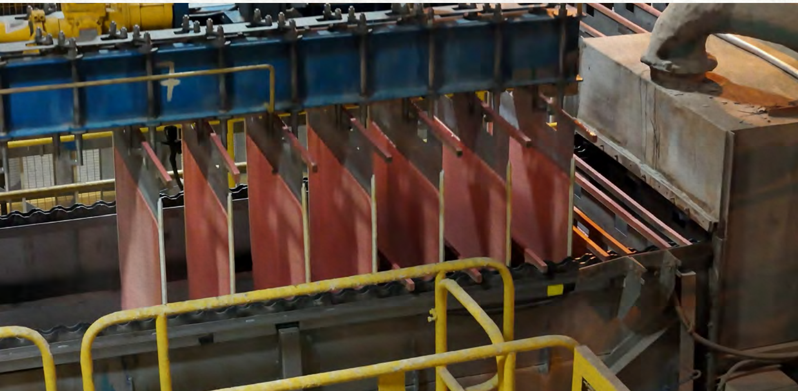
Mantos Blancos – Cathodes Collection at SX/EW Plant
